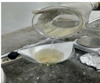
Fig 2: Filtering sample water (river water) using alpha cellulose
