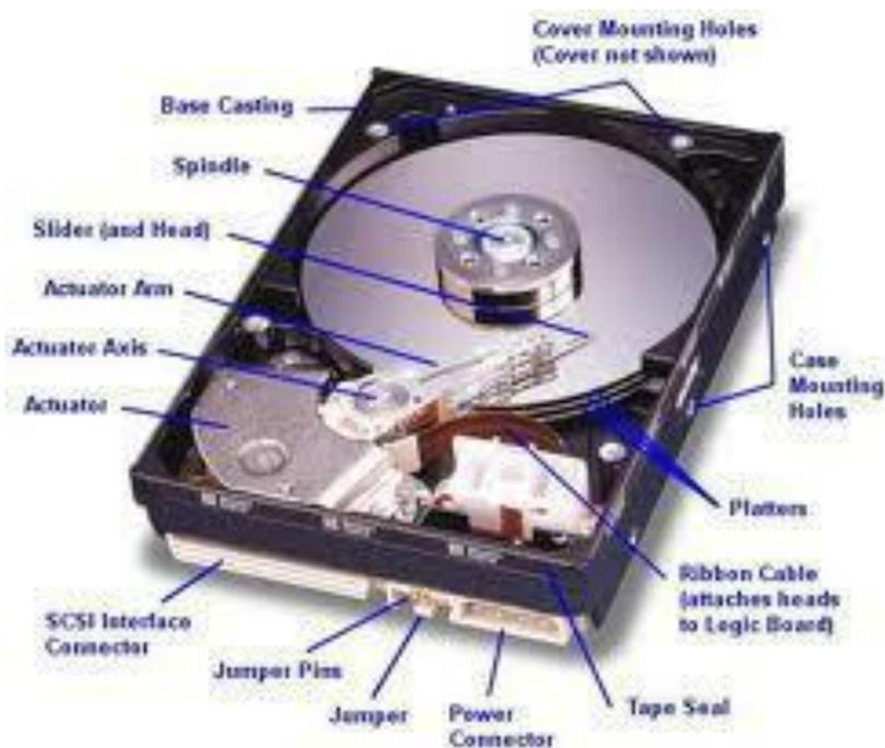
**Gambar 20.** Hard disk (<http://t0.gstatic.com/>)
