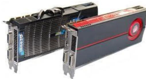
**Gambar 22.** *Graphic Card* (<https://encrypted-tbn0.gstatic.com/>)
