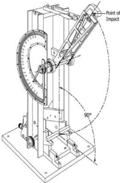
FIG. 1 Simple Beam (Charpy-Type) Impact Machine
