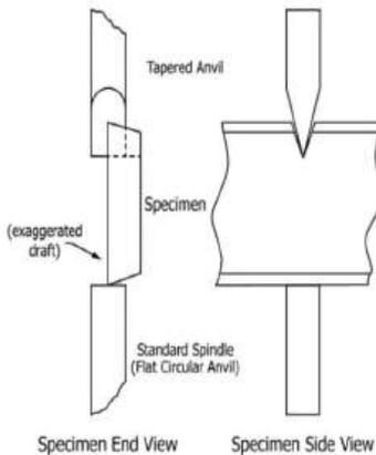
FIG. 5 Notch Depth Measurement on Test Specimens
