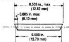
FIG. 1 Tension Test Specimens for Sheet, Plate, and Molded Plastics
