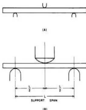
NOTE—(a) Minimum radius = 3.2 mm (1/8 in.). (b) Maximum radius supports 1.6 times specimen depth; maximum radius loading nose = 4 times specimen depth.
