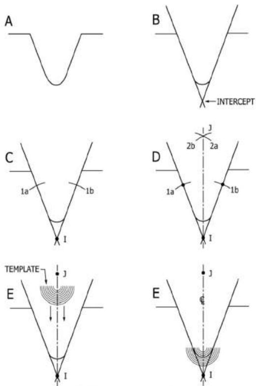
FIG. X1.4 Determination of Notching Radius
