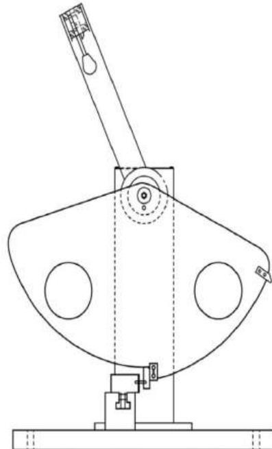
FIG. 2 Example of Compound-Pendulum-Type Machine
