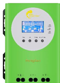
Gambar 2.3 Solar charge controller
