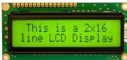
Gambar 2.11 Liquid Crystal Display (LCD)
