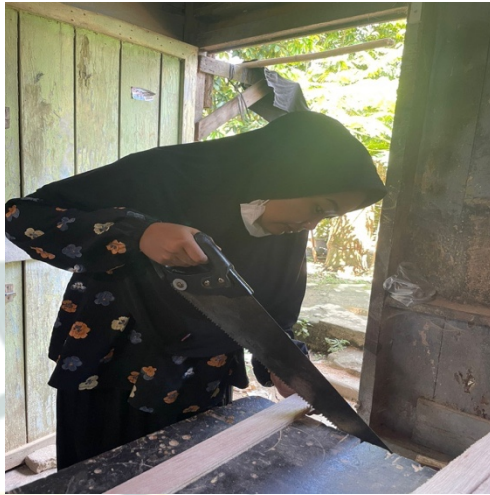
Gambar 2.2 Memotong Kayu Triplek
