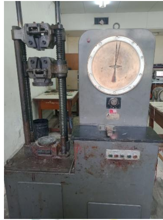
Gambar 2.10 Alat Uji Bending UTM (Unisversal Testing Machine)
