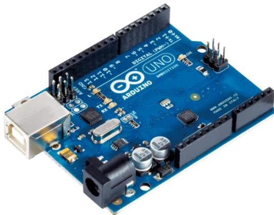
Gambar 2. 10 Papan Arduino UNO
