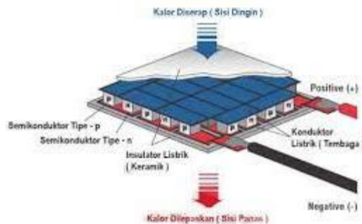
Gambar 2. 6 Skema elemen peltier (Agus Salim & Indarto, 2018)
