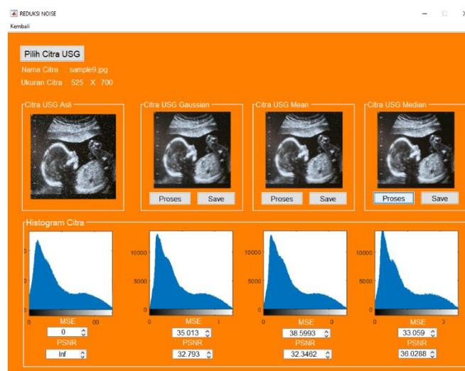
**Gambar 4.30** Citra USG sample 9 Reduksi *Noise Gaussian, Mean, Median*
