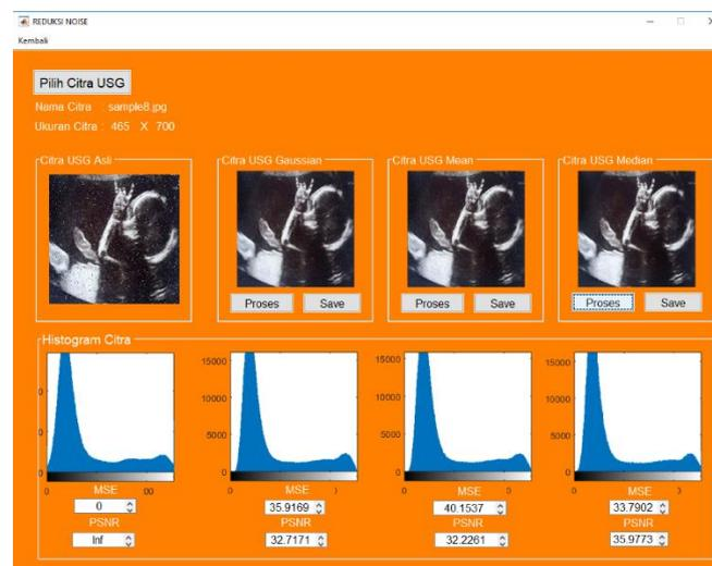
**Gambar 4.28** Citra USG sample 8 Reduksi *Noise Gaussian, Mean, Median*
