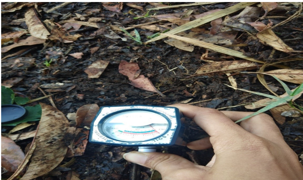
Gambar Pengukuran PH Tanah ( Soil tester )
